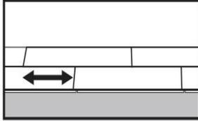
General: Minimum distance between short ends of Planks in parallel rows shall not be less than 400mm
