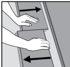
Disassemble the panels by sliding horizontally ! **Do not fold up !**
