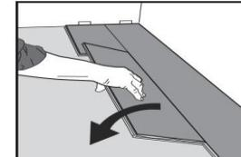
Fold down in a single action with a slight presto the short end of the previous. During fold down make sure the panels are tight against each other.
