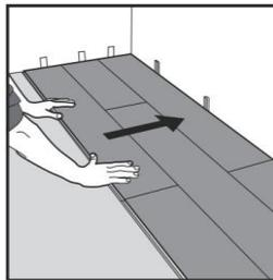
After 3 rows, adjust the distance to the front wall by placing distances abt 10mm to wall
