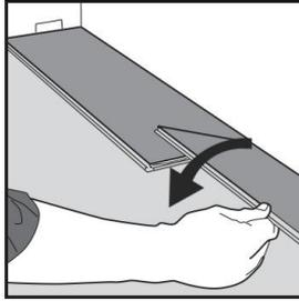
Place 2<sup>nd</sup> plank gently and tight to the short end of 1<sup>st</sup> plank. Fold down the panel down in a single action movement. During the fold down make sure the panels are tight against each other. Afterwards press or slightly knock at the short end just installed
