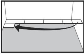
Second row. First plank minimum 500mm. Put a distance to the wall abt 10mm thick.
