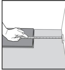
At the end of 1<sup>st</sup> row, put a distance abt 10mm to the wall and measure the length of the last plank to fit
